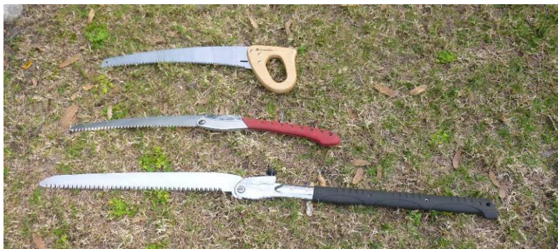
Japanese style pruning saws made by Corona (top) and Silky (bottom 2). The Japanese made saws are among the best available but the Corona is effective and cost much less.
