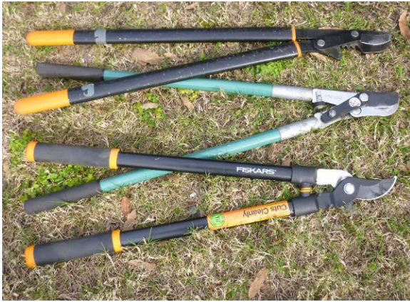
Bypass loppers. Simple (bottom), compound lever-action (center), compound gear-action (top)
